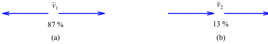
Figure 6.3: In the simplest case of two beads oscillating on axis [i.e. (\theta_1, \theta_2) = (0, 0) ], the two normal modes of oscillations \tilde{v}_1 and \tilde{v}_2 are simply antiphase motion (a) and in-phase motion (b). The geometry of the modes is illustrated by the vector pairs \tilde{v}_1 and \tilde{v}_2 ; the eigenvectors are labelled from 1, \dots, N (in this case N = 2 ) in order of decreasing relaxation time scale, and this convention is followed throughout this chapter. The percentage indicates the fractional amplitude observed experimentally from the decomposition of the steady state solution onto the normal modes, as defined in Eq. (6.16).
